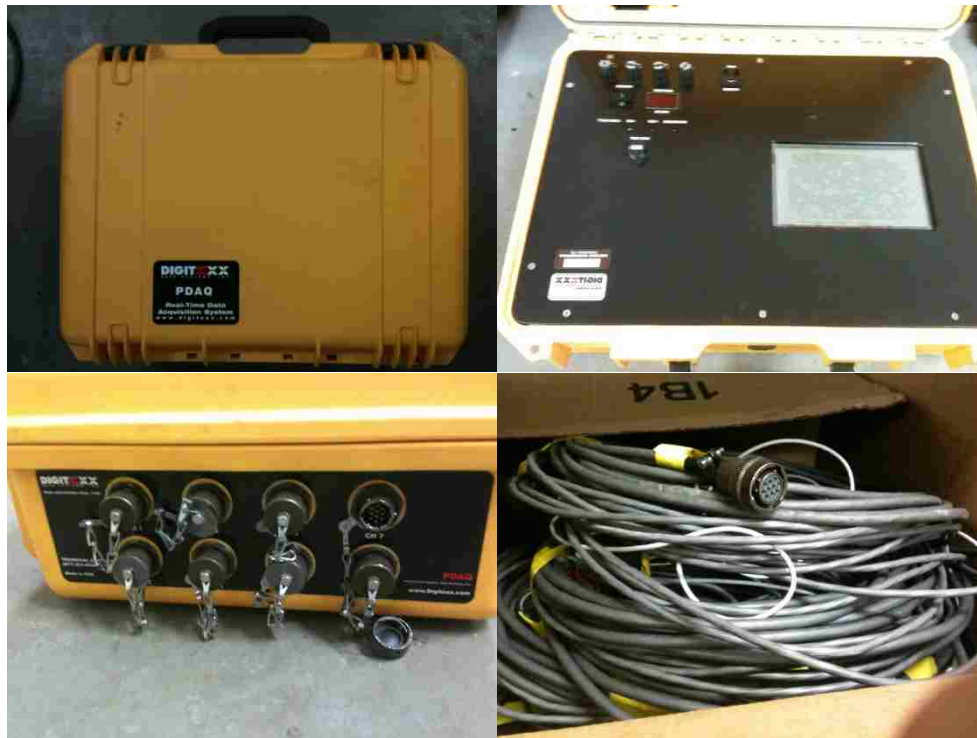
Figure 2.5 PDAQ Digetexx data acquisition system with the connecting wires (last plot)
