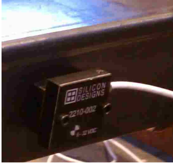
Figure 2.3 Silicon Designs wired sensor, mounted on a steel tube (courtesy of Ms. Elizabeth L. Labuz)
