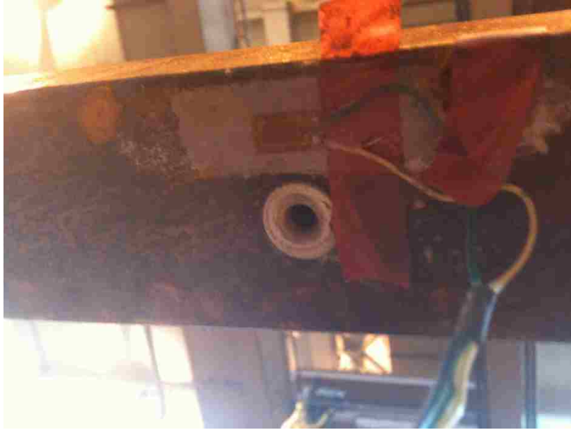
Figure 8.1 strain gage model CEA-09-250UW-120, instrumented on the 2-bay frame
