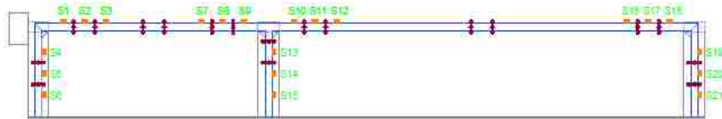
Figure 5.5 A schematic plot of the girder mounted with accelerometers
