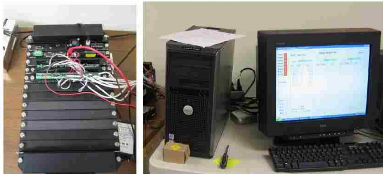
Figure 2.6 CR9000 data acquisition system: wire jack and user interface
